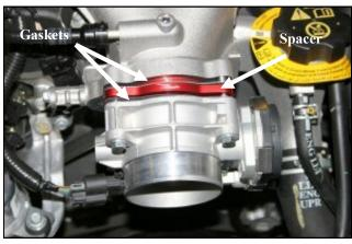
4. Install the Poweraid Spacer between the throttlebody and the intake manifold with the first supplied gasket next to the intake manifold, and the second supplied gasket next to the throttlebody as shown. Make sure the "flow" arrow printed on the spacer is pointing towards the intake manifold.
